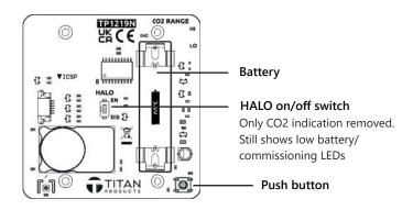
The sensors are supplied with a battery tab in place. Remove this before attempting to commission the device.
