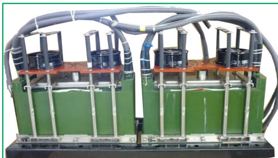
Dual Transformer w/ Pulsed Ventilation Ferrite U126 Cu Foil Technology 125 kW @ 4 kHz 500 V / 940 V 1132 x 348 x 500 mm 190 kg Railway Application
