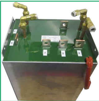
Transformer 120 KW @ 20 KHz P: 720 V (Square) S: 1500 V (Square) 350 x 300 x 300 mm – 62 kg Cu Band Winding, Ferrite U126 Core Industrial Coating Machine Application
