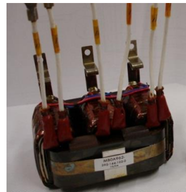
Autotransformer 22,5kVA 115V @ 400Hz 110x75x90 mm Aluminum Foil , C-Core technology Aerospace application (thrust reverser)
