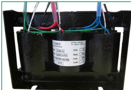
Twelve Pulse Autotransformer 200V/400V 2KVA @ 400Hz Cu Magnet Wire, SiFe Laminations 125 x 70 x 88 mm – 1.7 kg Avionic application
