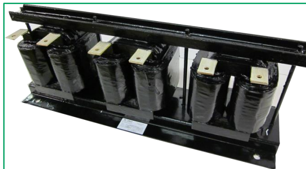
3 x inductances – 70 \mu H 200 A @ 400 hz/ ripples 20 A @ 10 khz Cu Foil winding, AMCC Core 500 x 150 x 200 mm - 24 kg Ground Power for Aircraft
