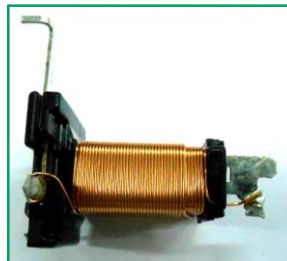
Primary Coil 38 x 22 x 24 (mm) Automotive application
