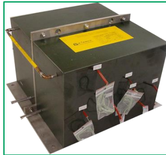
Transformer 2x75 KW @ 18 KHz P: 678 V S: 800 V 350 x 300 x 300 mm – 62 kg Cu Band Winding, Ferrite U126 Core Industrial Coating Machine Applications
