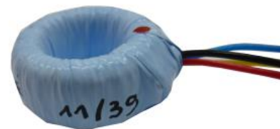
Current Sense Transformer 75 A / 45.4 mA @ 720 Hz ø 26 x 13 mm 16 g Class H Nanocrystalline Tape-wound Toroid Aerospace Application
