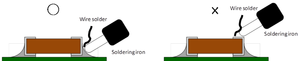
Fig 3 Correct handling method of soldering iron
