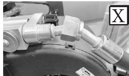
Improperly Seated O-ring Land
