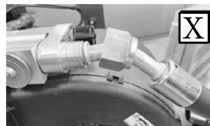
Improperly Seated O-ring Land
