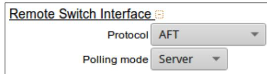
At the scheduled poll events, any new files deposited by the switch are processed and placed into the file forwarding subdirectory for transfer to the billing/mediation server.
