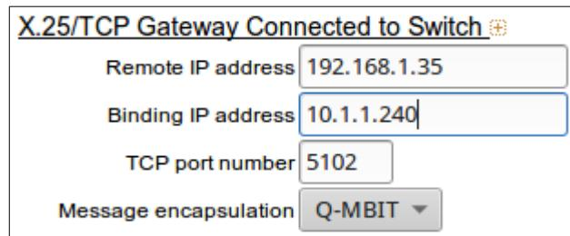
The local or remote X.25 Gateway must be configured to listen for the incoming X.25 connection, and the TCP/IP destination must match these parameters. For example, the Microtronix X.25/TCP Gateway:
