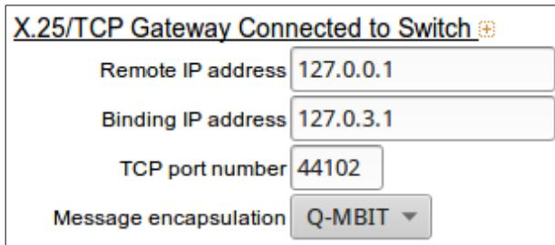
The **Remote IP Address** is set to the address of a local or remote gateway which connects directly to the X.25 interface of the switch via a WAN interface. The **TCP to X.25 Routes** section of the gateway must listen on the **TCP port number**.
