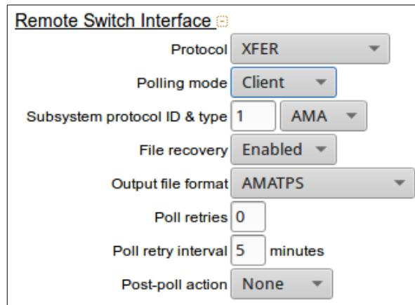
The **Protocol ID** field must be set to a non-zero value to collect files and must correspond with the subsystem value expected by the switch for the type of file collected. The **Protocol Type** field must be set to the type of file. This should correspond with the subsystem ID type on the switch..
