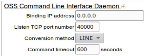
Select the TCP port number [and binding IP address] on which the CLI interface listens for TCP connections from the remote terminal emulator. A server daemon is started that waits for a user to connect, then connects to the AXE's command line interface via the X.25/TCP gateway defined below.
