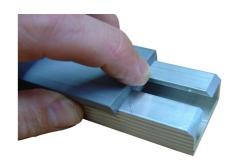
When butting two sections at right angles, chamfer the top corner of the aluminium extrusion to allow for the polymers to butt together neatly
