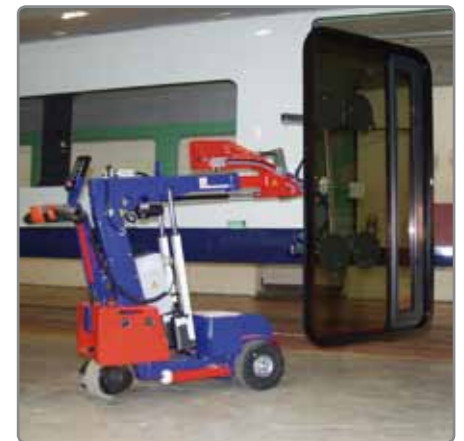
KS Robot 280 at the assembling of doors in German ICE trains.
