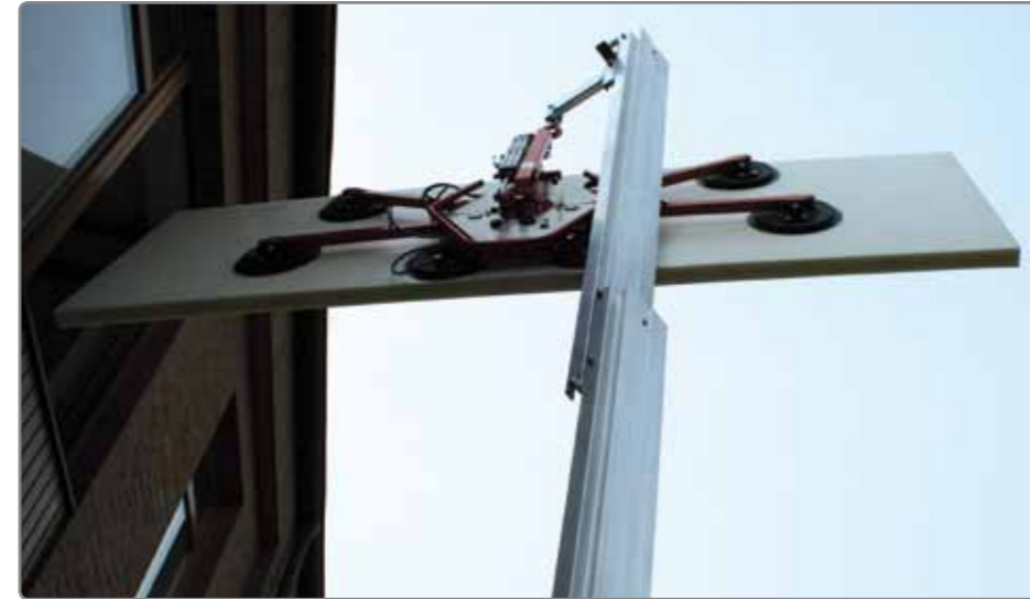
Mast with hook adapter for supporting of a lifting belt or a suction unit.
