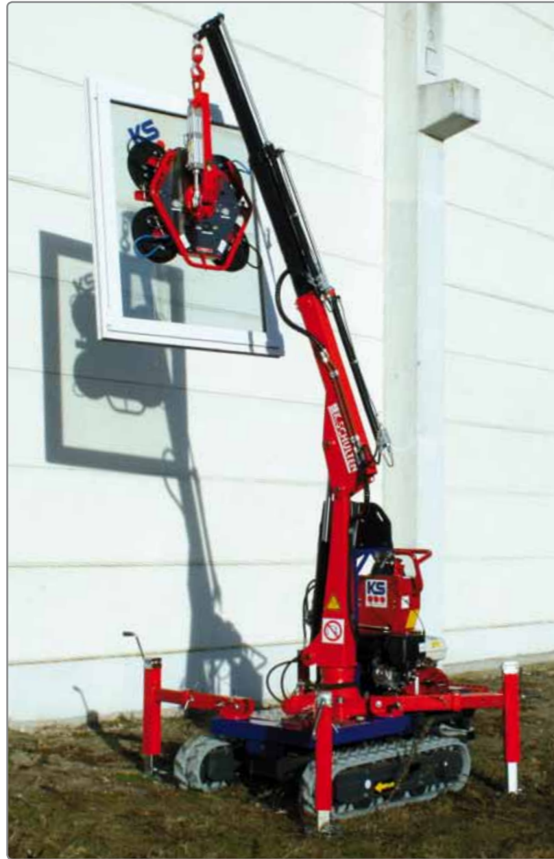
KS MultiCrawler C500 is equipped with a KS VacuPower suction device*, ideally suited for lifting of glass panes, wood and stone plates, pvc black boards, iron sheets and further more bulky goods.
