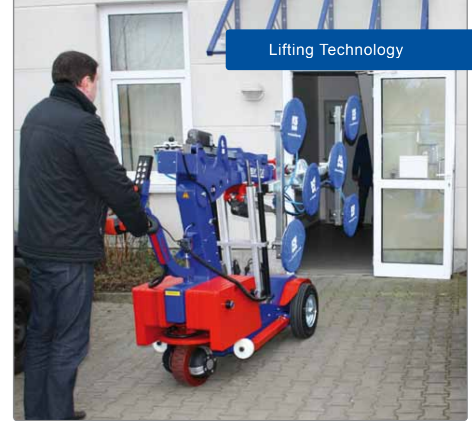
Very articulated: 90° slewing unit slews the suction device lateral for driving through small entries.
