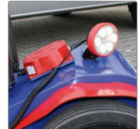
LED lamp* makes it possible to work in the later hours.
