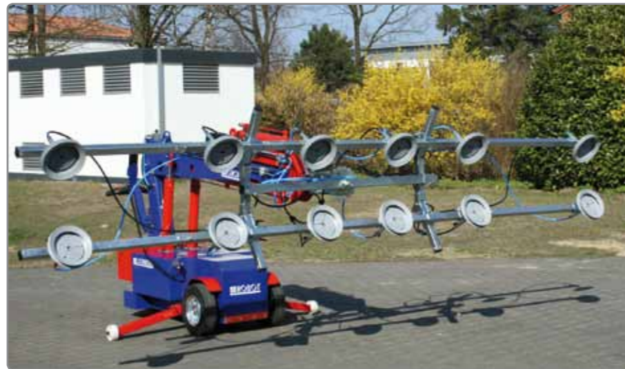
KS Robot 1000 with vacuum suction unit for curved glass*.
