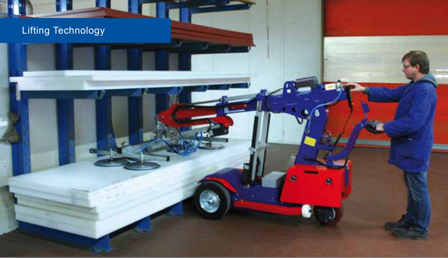
First class: electrical buckling link hinge makes the loading from heavy plates directly from the shelf possible.
