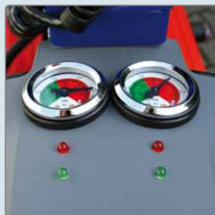
Display shows the power of the suction unit and warns you in case of vacuum loss.
