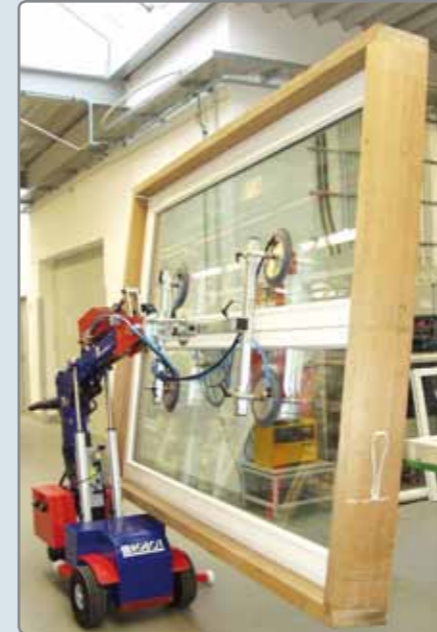
Sideward swing function for the transport through small ways.
