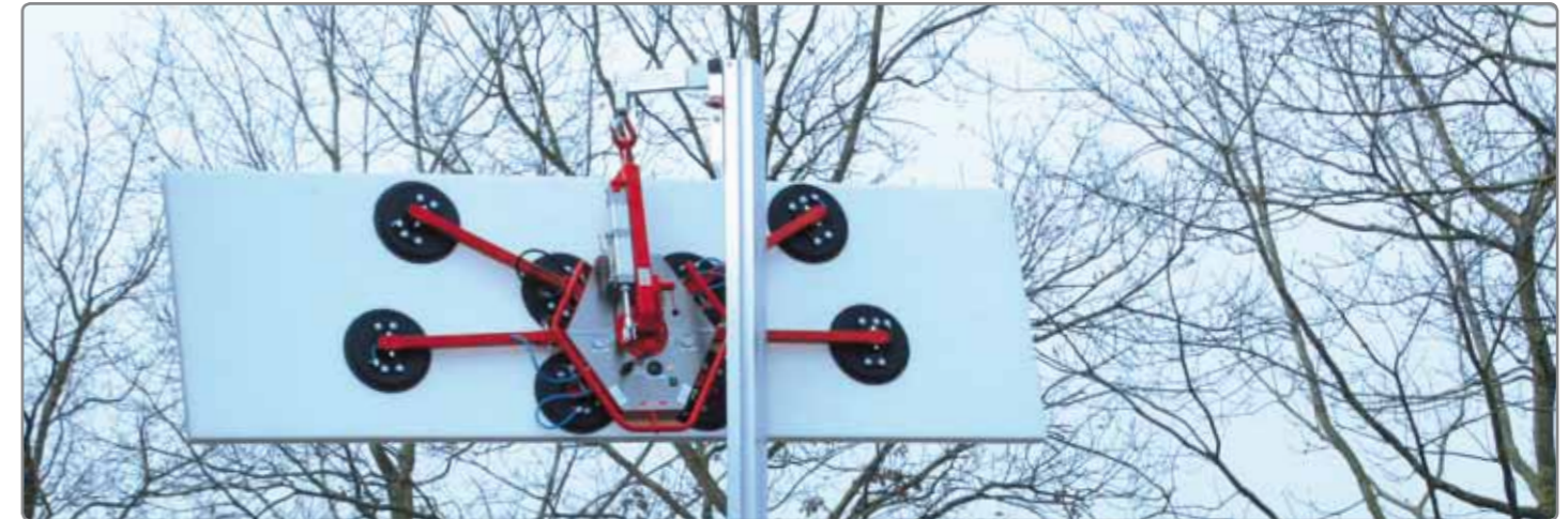
KS vacuum suction unit for elements up to 600 kg.
