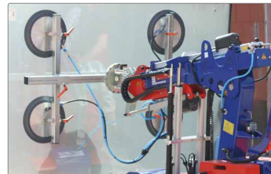
Equipment with special turning articulated joint* makes the installation easier: all turning and tilting movements are controlled electrically.
