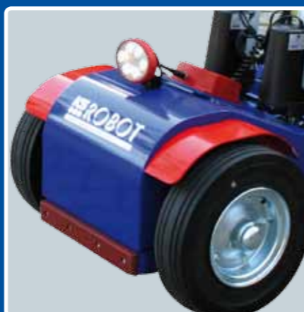
Solid rubber tires with a wide surface even when increasing.
