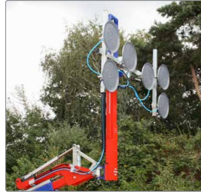
Extension of telescopic* for all KS Robots, limited to a load capacity of 250 kg.
