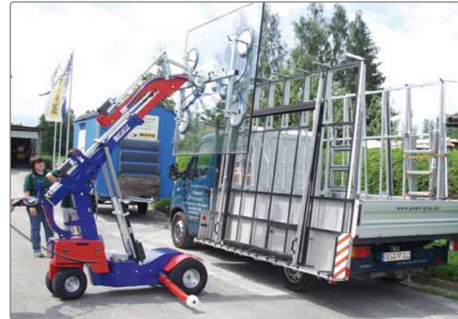
KS Robot 600 Offroad during loading of glass panes.
