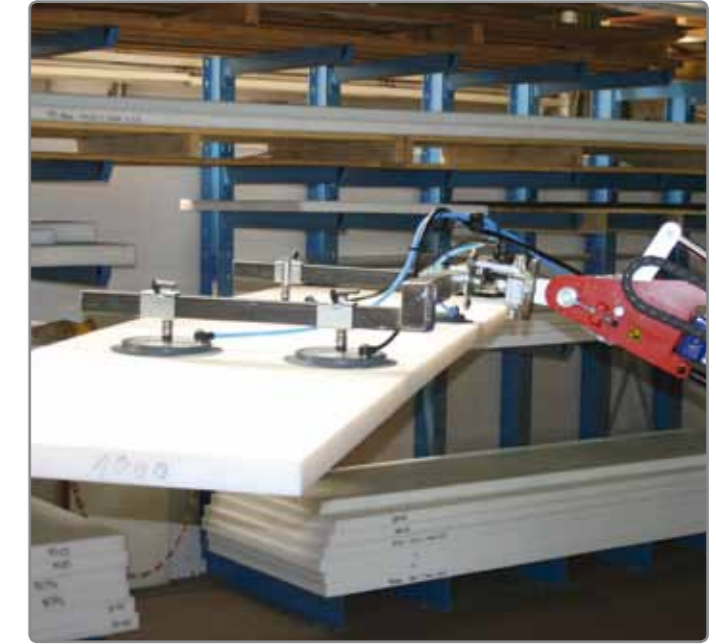
Special fork* takes the plates out of the shelf with a low height.
