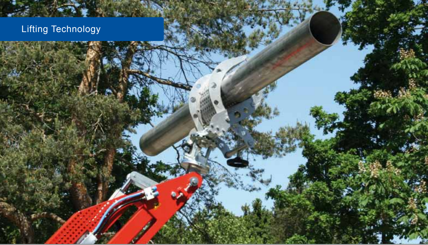
Special gripper for carpets or metal tubes possible electrically and mechanically.
