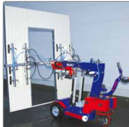
Ideal: vacuum suction load with thin suction* for trapezoidal plates.
