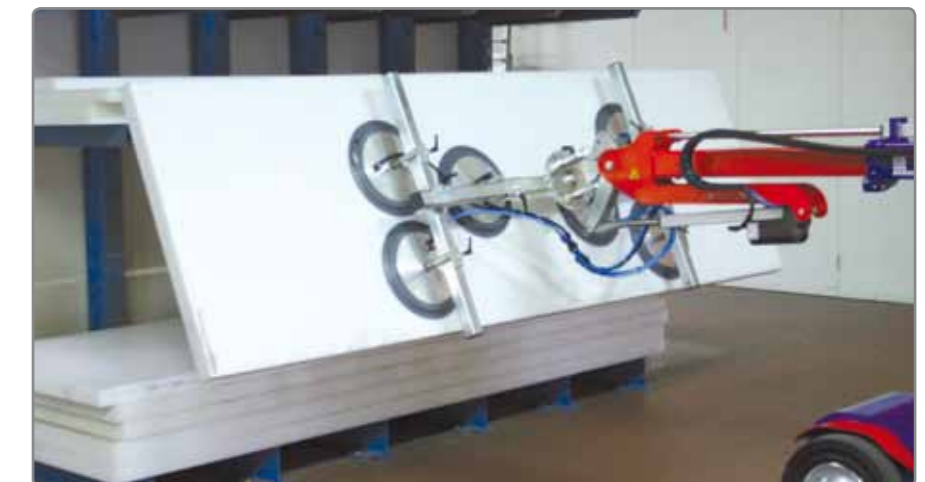
The Robot can take heavy plastic plates of 600 kg out of the shelf, put them on a pallet and swing them overhead*.
