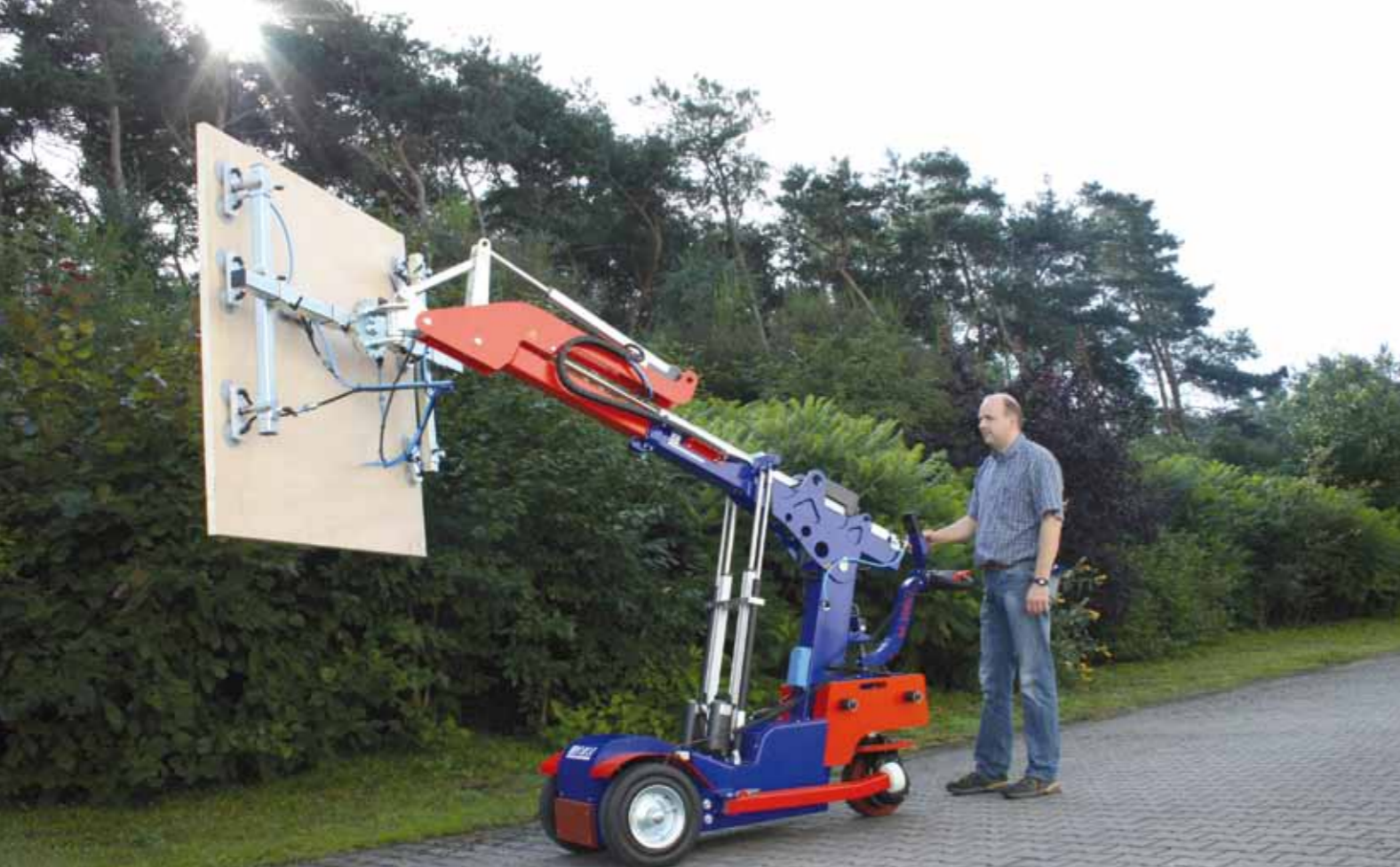
KS Robot 400 with a special vacuum suction unit for plates made out of wood.
