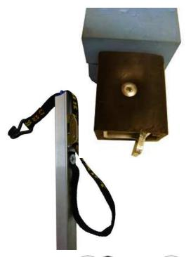
The top cleat is part of the structure and allows the hook on the strap pole to easily connect to the structure. For hardtop vehicles a pin top pole and locator is used.
