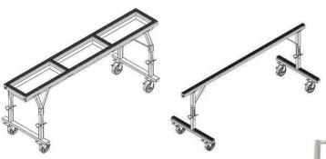
Assembly and glazing tables with non-marking polymer work surfaces to avoid swarf damage to window frames. Optional tilting function to allow semi-vertical loading, unloading and glazing as well as lying flat for fabrication. Access to the window frame from both sides to aid fabrication
