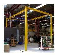
Light freestanding overhead crane systems for loading and unloading, and moving packs up to 1000kg around the factory
