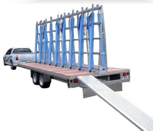
The Glass Racking Company fixed A-frame window trailers have been designed to transport the increasing size and weight of modern window frames and double glazing. The trailers are built to utilise the The Glass Racking Company Window Retention system to speed load and unload times and reduce rework resulting from transit damage to glass and window frames.
