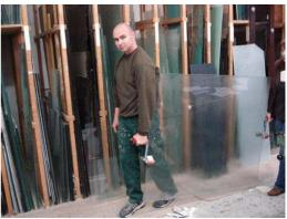
The Glass Racking Company supplies the Australasian market with Carrymate Transport Grips. These clever lifting handles ease the effort required to lift heavy loads, reduce injury, and are suitable for lifting a range of flat sheet products including window frames, sheet glass and DGUs.
