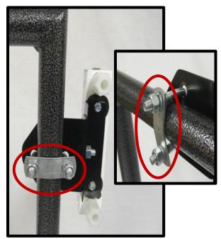
The FM-1008.5-LED Flowmeter should be mounted outside the cab in a location that is easy to view for the operator. Find a desired location to mount the FM-1008.5-LED Flowmeter.
