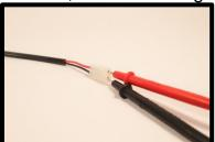
Voltage reading must be between 10-15 volts.
