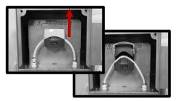
**4.** To open the pump head, lift up on the front of the hinged pump head.
