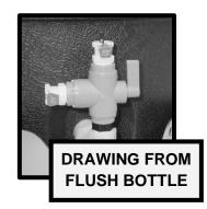
1. Even if the cooler is empty, a good habit to get into is start by turning the cooler valve off. When off, the valve handle will either be facing out towards you, or up towards the line from the flush bottle.
