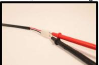
Voltage reading must be between 10-15 volts.
