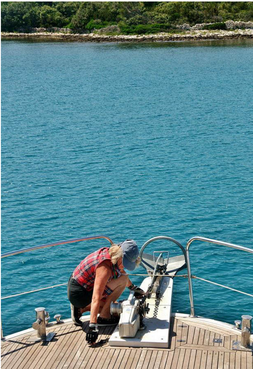
Securing the anchor back on deck
