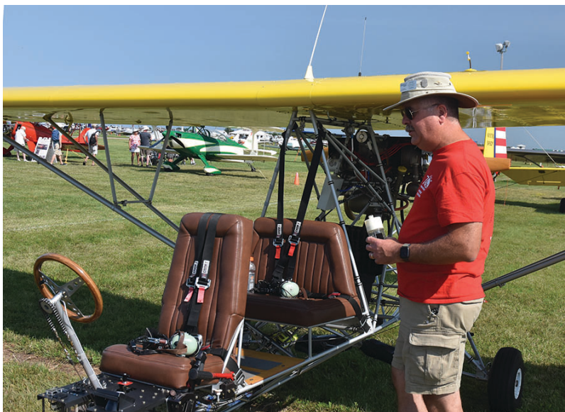
Jeff Point is a retired Milwaukee police captain with a passion for flight. His favorite homebuilt is this flying skeleton called a Breezy; the lattice-like structure is light-weight but incredibly strong.
