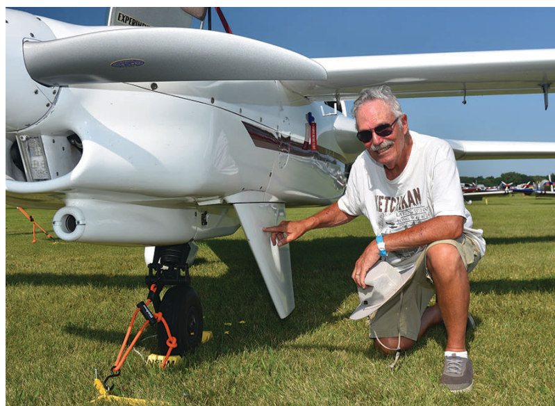
The Defiant is a home-built version of the venerable Cessna 337, a twin-engine speedster with center-line thrust. The design is odd in many ways, including the unique "rhino rudder" at the front of the airplane, below the cowl.
