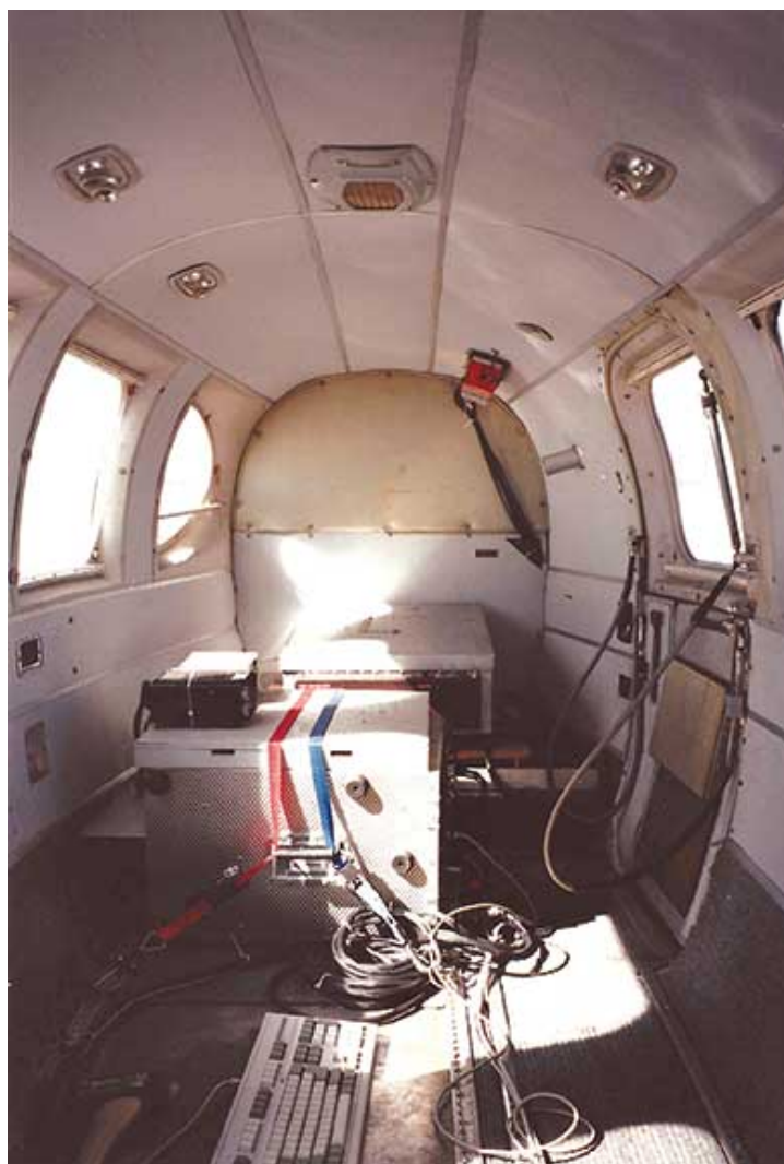
The back of the Navajo was relatively cavernous, holding the GPS-based survey computer and the magnetometer system which protruded behind the tail of the airplane similar to the Navy's P3 subhunters. (The magnetometer was so valuable to engineer took it home every evening and slept with it under his pillow.) This spacious cabin was nearly the undoing of Vince and Franco as they flew their final mission.
