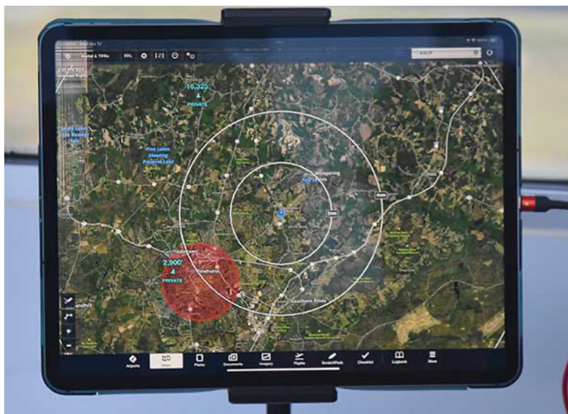
The ADSB system in the control tower is used for awareness but not for IFR control procedures. Notice the red circle denoting a TFR over the actual tournament. A Cessna 182 hired by the USGA circled over the tournament every day, taking photos.
