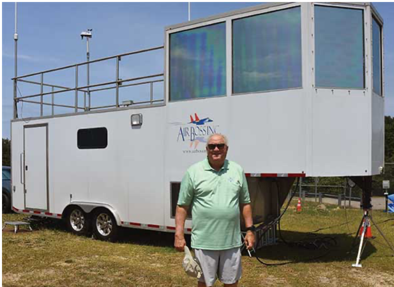
George Cline shows of his one-of-a-kind mobile control tower, built on a frame similar to that which would be used for NASCAR racing teams or a large horse trailer. The system is towed behind a massive Ford F450 pick-up truck. The lower portion is an office and breakroom; the raised tower is on the right, and the open upper deck is used for airshow commentators.
