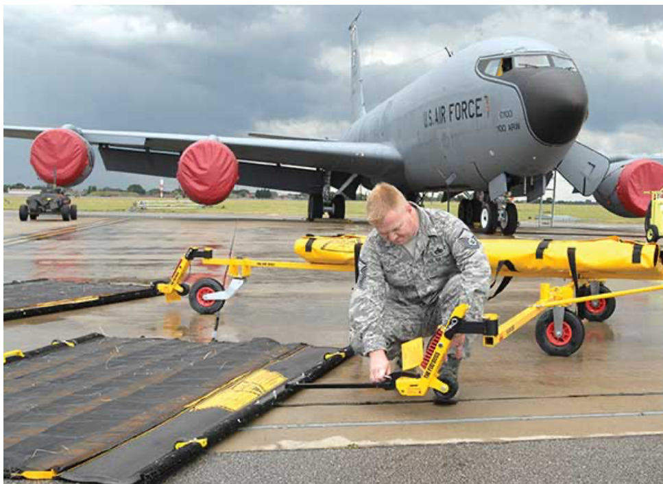
FODBoss systems are in use on all six continents, by many major airports, and by military operators as well. The USAF keeps FODBoss systems running on all of their fields not just to protect their expensive aircraft but also to avoid damage to radar-defeating stealth coatings found on the F-22, F-35 and B-2 aircraft. Shown here: a technician prepares to tow a FODBoss in front of a KC-135 tanker aircraft.
