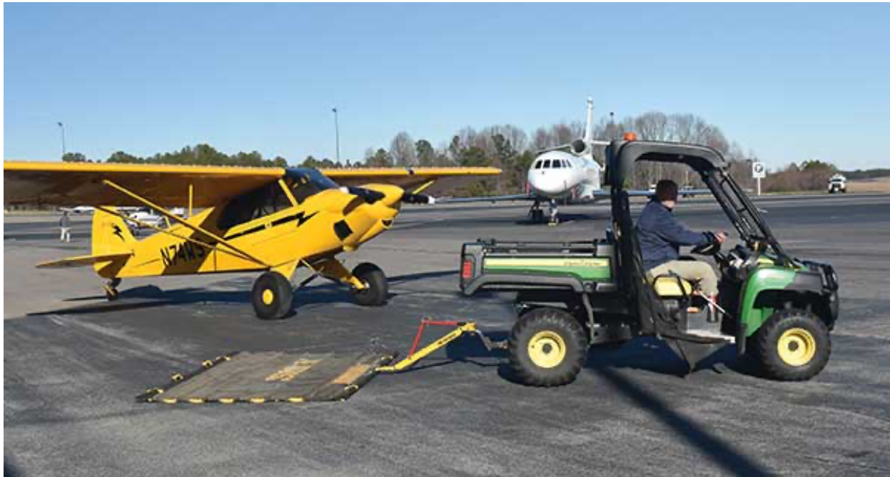
Paul Puszyński, the Ops Manager at the Pinehurst/Moore County Airport in central North Carolina, demonstrates the ease with which a simple utility vehicle (or even a golf cart) can tow a FODBoss on the ramp. For the runway, they usually use a truck. A FODBoss is effective up to 40 mph, so runway sweeping behind a pick-up truck is faster and returns the runway into service more quickly than when using a smaller vehicle.
