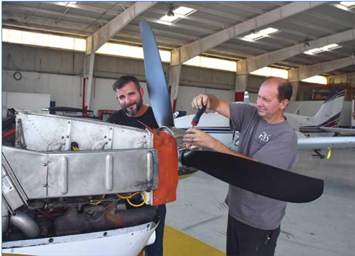
Out with the old, in with the new. Here Brandon Smith (left) and Steve Brown from Pinehurst Aviation Services finish installing the new Hartzell scimitar prop on to the nose of 7591N. It does look sexy... Jonesy can't wait to see how it flies.
