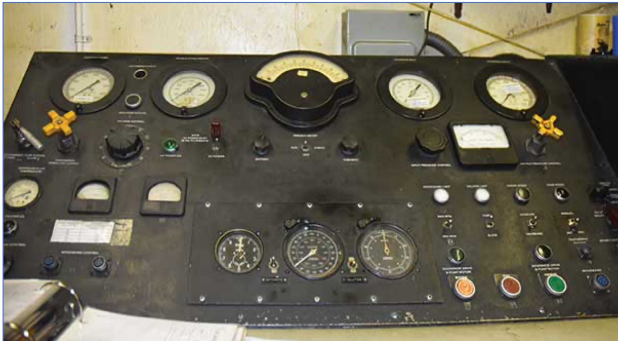
This large system is a simulator to test the performance and the precision of prop governors. Martin asserts the constant-speed prop governor is the “hardest working part on an airplane.” This simulator, despite its obvious age, can put a governor through more stress than it would ever see in flight, so H&H can be comfortable the machinery will work as advertised.
