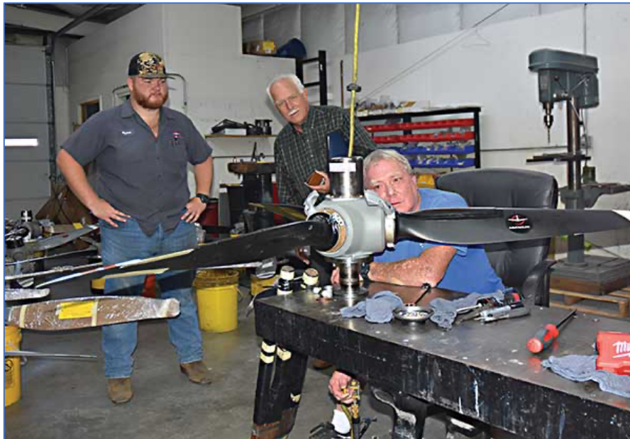
The H&H lab is able to put prop systems through all of the required tests before being returned to the field. In this case, Martin is boosting the oil pressure inside the hub of this constant speed prop to see if the blades change pitch as they should. Notice his right hand is below the workbench, turning the valve that controls the flow of oil. This is the same function the prop governor performs on the plane in flight. John “Raynor” Wiygul and Jonesy watch as Martin moves the blades slowly and silently, almost magically, back and forth.
