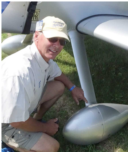
Greg Buller is an AirVenture Homebuilt judge and knows RV aircraft can develop a tear in the aluminum wheel fairings; here he inspects one fairing looking for a strain-release design.
