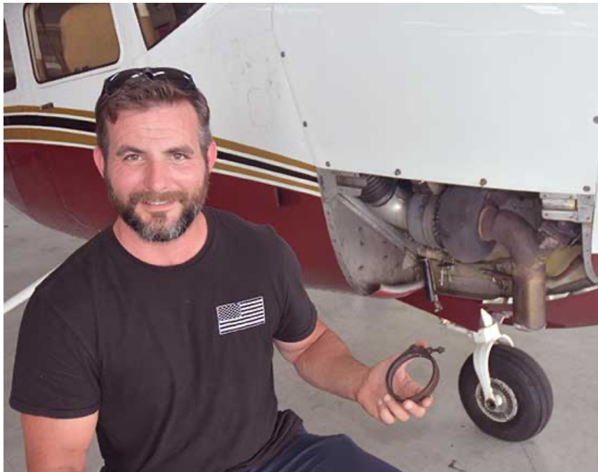
Brandon Smith is a brilliant A&P at Pinehurst Aviation Services at the Pinehurst (Moore County) Airport in North Carolina (KSOP). The V-band clamp in his hand just came off the turbocharger on my T210 behind him. Smith performed the seven inspections required by the new airworthiness directive and found the clamp failed three of the tests. This particular part may have had as many as 1,700 hours in service.
