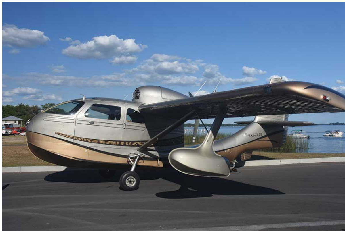
This handsome Republic Seabee is a classic seaplane amphibian. The fuselage of the plane itself is designed with the hydrodynamics and strength required of a high-speed motorboat. Notice the top-mounted, rear-facing engine which keeps the prop away from the erosive effects of water spray.
