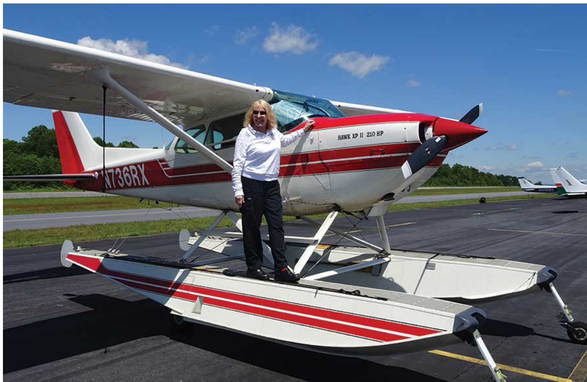
Susan VanFleet flies N736RX, a bright Cessna 172K with a six-cylinder, 210 hp Continental IO-360K turning a constant-speed prop. Since the original C-172 only had 145 hp one doesn't have to be an aerospace engineer to predict exciting performance from Susan's red and white beastie.
