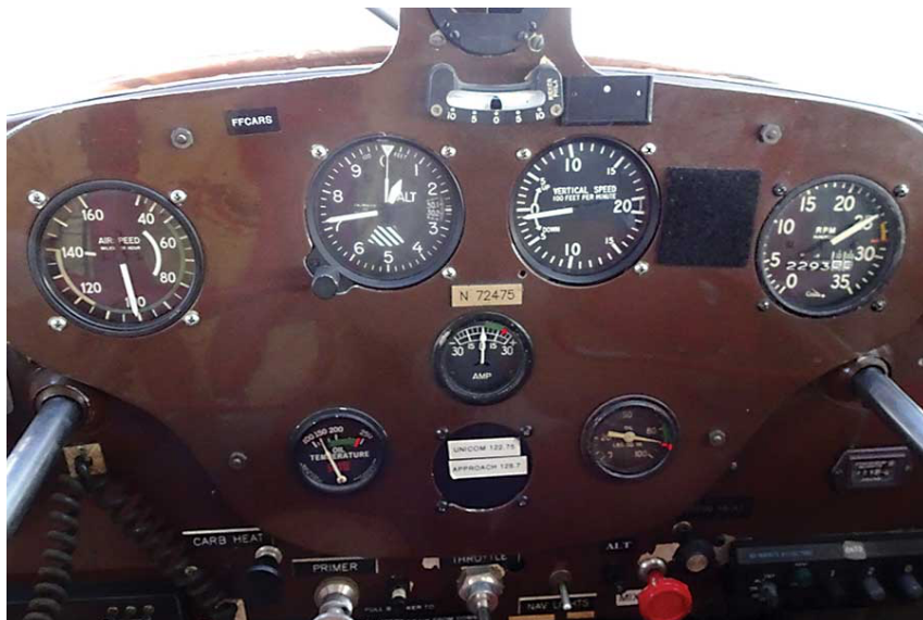
The panel of the Cessna 140 is vintage VFR Cessna engineering. We're level at 700 feet over Lake Dora, motoring along at 100 miles per hour, cranking about 2500 rpm on the little Lycoming engine. In this age of flat-screens and magenta lines, simplicity is heart-warming.
