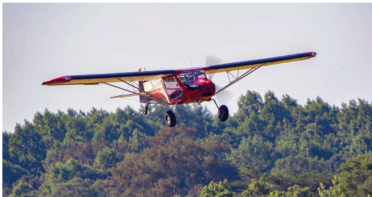
The Bushcat has a low wing-loading, which means relatively few pounds of airplane for each square foot of wing. This makes the plane vulnerable to gusty winds and pilots should always be ready to trigger-ready for the "go-around" decision.
