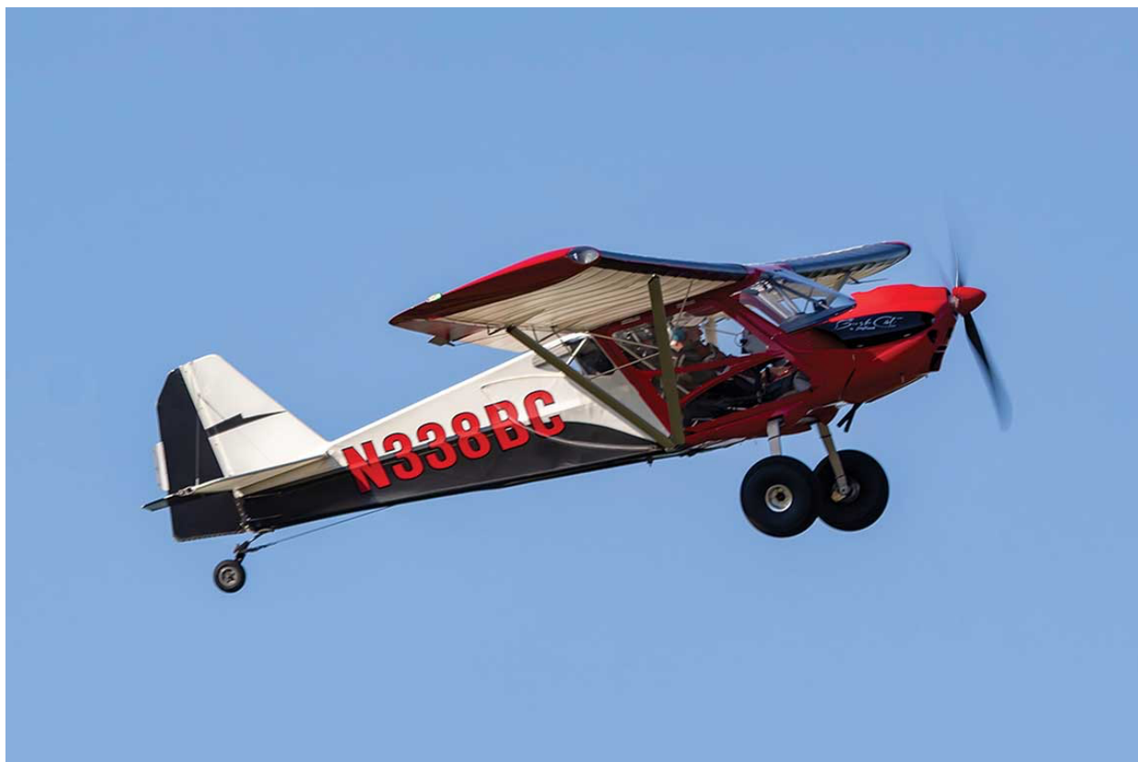
The Bushcat light sport airplane is a joy to fly. It's a two-seat taildragger with side-by-side seating, which is a rarity. The plane is available in a nose-wheel configuration
