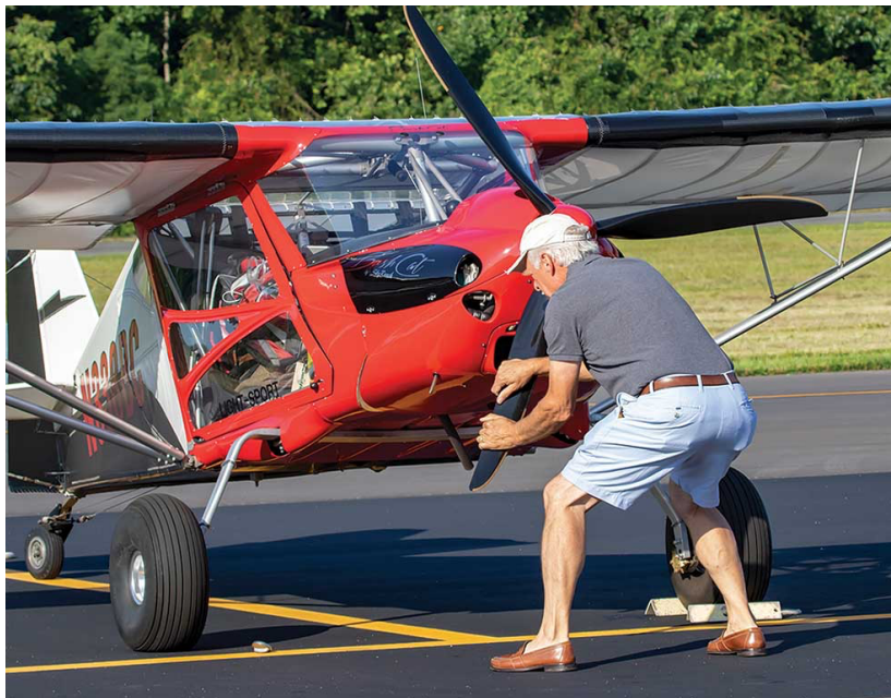
Rotax operators will recognize this position: the author is “burping” the oil system in the engine. After 15 or so pulls on the prop the engine releases a flatulent gurgle of oil, which means the system has been pre-lubricated and is ready for start.
