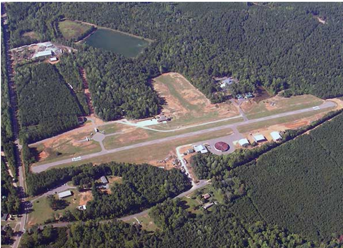
Gilliam-McConnell Airport in Carthage, NC. Notice the round hangar? The entire building spins and pivots on a massive center post, allowing eight or nine planes to share just one single door. Across from that hangar is the award-winning Pik-n-Pig restaurant. It burned a few weeks after this photo was taken and has been rebuilt; COVID slowed the re-building process but it should be re-opening by the time your read these words.
