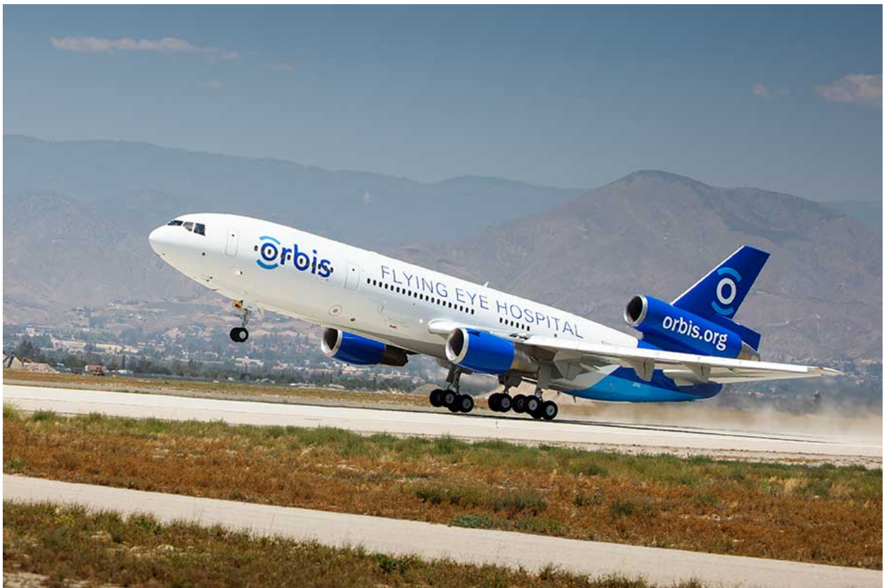
The Orbis flying eye hospital is a giant MD-10 cargo hauler made in 1973 that has been modified to carry a completely self-sufficient operating room, patient care facilities and medical training systems. It travels the world delivering eye care where it is needed most. Photo by Paul McKelvey.
