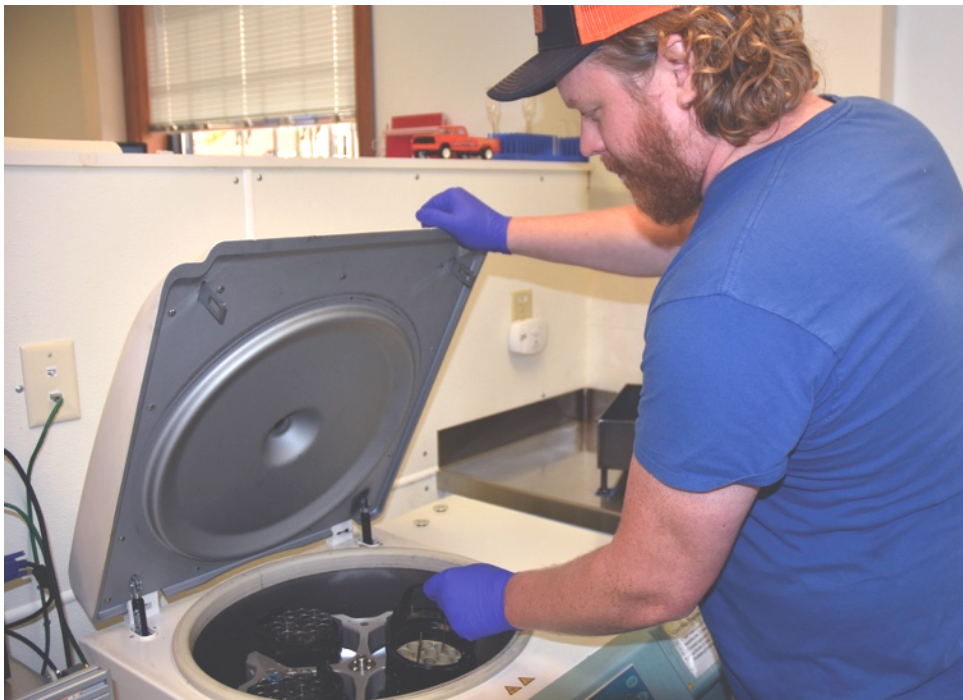
Luke inserts the samples into the centrifuge system which spins them at 2,000 rpm to separate the particulates from the oily liquid. These particles are so small they are not captured by a traditional oil filter. Subsequent spectrographic analysis determines the composition of the residues which helps with diagnostics.
