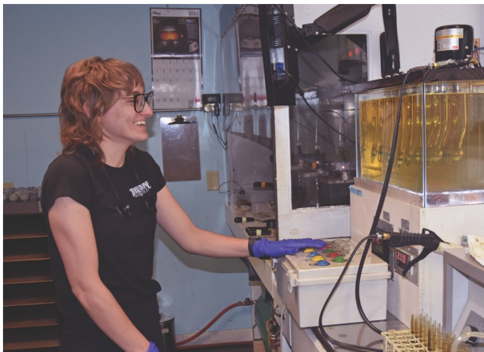
Lydia works all day in the dimly-lit flashpoint lab. Lydia is one of the many lab techs working at Blackstone. She is monitoring the kinematic viscosity bath which measures the viscosity of the oil; behind that is the flashpoint testing bay.
