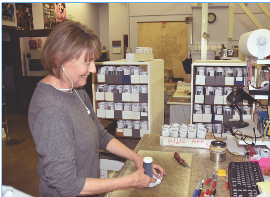
The volume of samples racing through the Blackstone facility is amazing to see, but each sample gets personalized handling and tracking every step of the way. Here, Mary unpackages an incoming oil sample and categorizes it by the source: aviation, diesel, marine, and so on.
