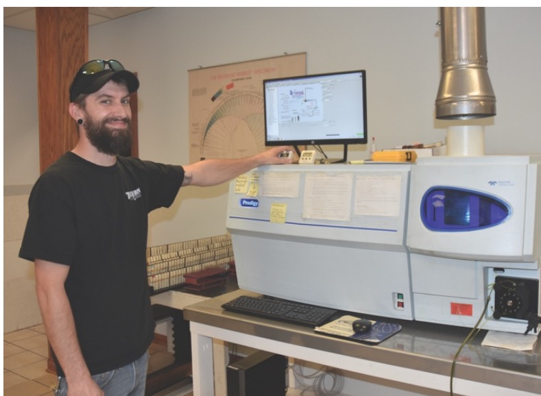
Justin poses with one of Blackstone's three spectroscopy machines. The digital spectroscopes heat the oil samples to determine the presence of twenty different elements which are tracked to measure engine performance. At this moment, Justin was recalibrating the machine, a task they perform every dozen samples just to be sure their samples are pin-point precise.
