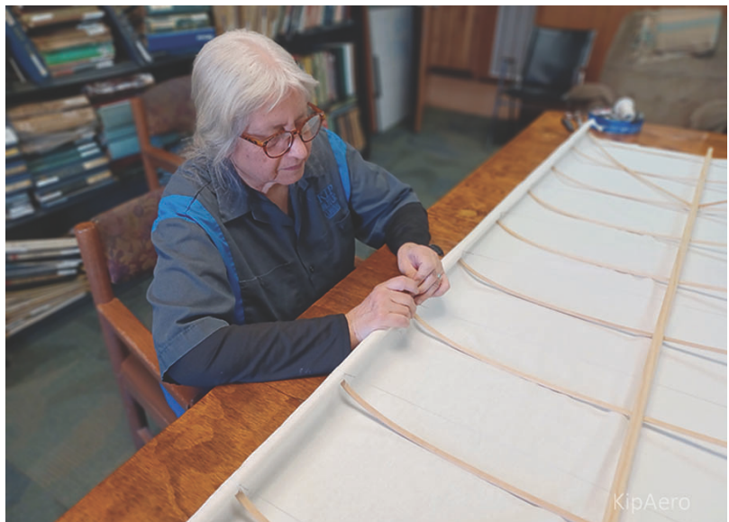
The Kip Aero team made dozens of spars and ribs for the four wings and the tail, then carefully hand-stitched China silk on to the fragile structure.
