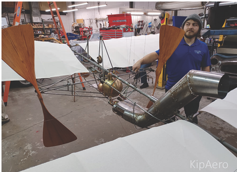
The aerodrome completely assembled, showing the engine and the exhaust. Notice how the engine components are integrated into the fuselage itself; this is a common characteristic of steam engines.
