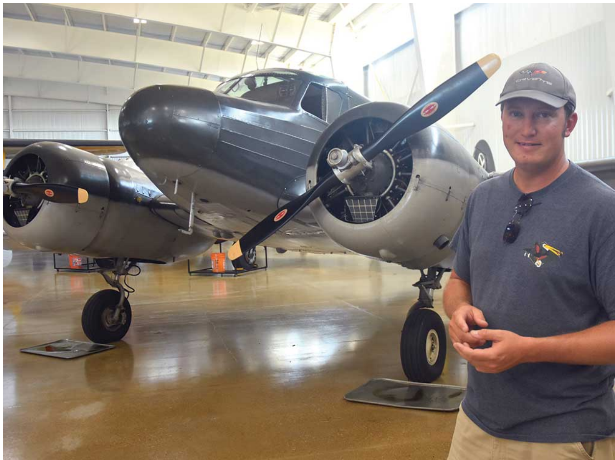
Andrew Kiest stands in front of the Museum's AT-17 Bobcat. This twin-engine trainer was designed and manufactured by Cessna during World War II to bridge the gap between single-engine trainers and complex, powerful, twin-engine combat aircraft. The wing is made of laminated spruce beams with plywood ribs, which led to the moniker the "Bamboo Bomber." It cruised at 150 knots and had a range of 650 nautical miles; about 5,500 units of the five-seat plane were built. Cool piece of trivia: this model plane was featured in the television series "Sky King."
