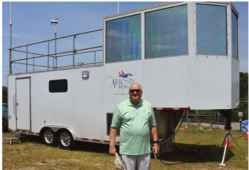
George Cline shows of his one-of-a-kind mobile control tower, built on a frame similar to that which would be used for NASCAR racing teams or a large horse trailer. The system is towed behind a massive Ford F450 pick-up truck. The lower portion is an office and breakroom; the raised tower is on the right, and the open upper deck is used for airshow commentators.
