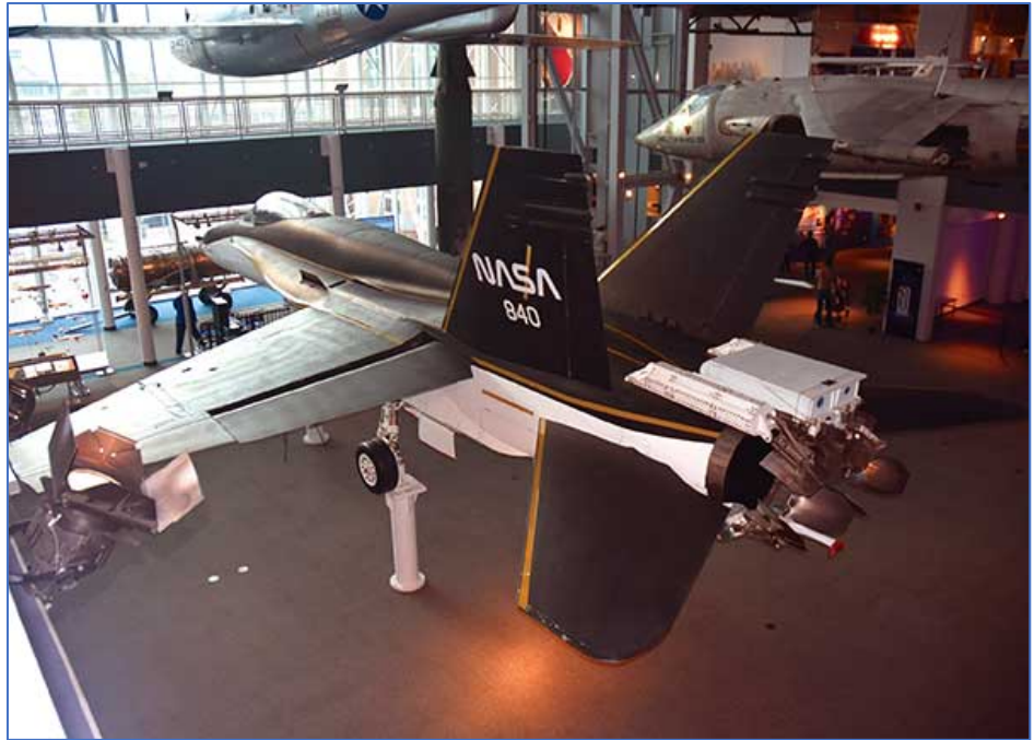
This highly modified F-18 was used by NASA in the development of thrust vectoring technology, which increases the agility of an airplane. The early thrust-vectoring equipment can be seen at the back of the aircraft.
