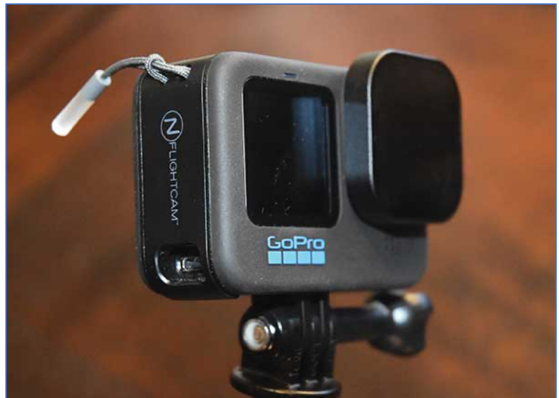
On this GoPro 10 camera, notice the NFlightCam replacement battery cover. This hatch voids the waterproofing of the GoPro 10 but allows access to the micro-USB port. With access to that port you can power the camera or record intercom audio, depending upon the cables you employ.
