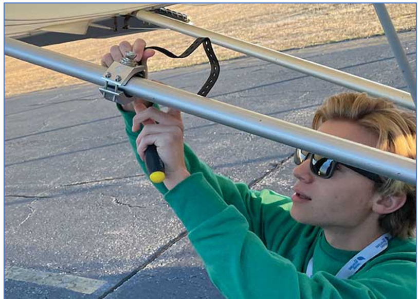
My favorite GoPro mounting system for airplanes with struts. Made of heavy aluminum, this clamp firmly grips the strut without damage to the structure or the paint. The lengthy strap allows it to fit struts of any size. A rock-solid design from NFlightCam. In his left hand, Chris is using the hex-head screwdriver to tighten the fittings on the clamp. That is one very clever innovation.
