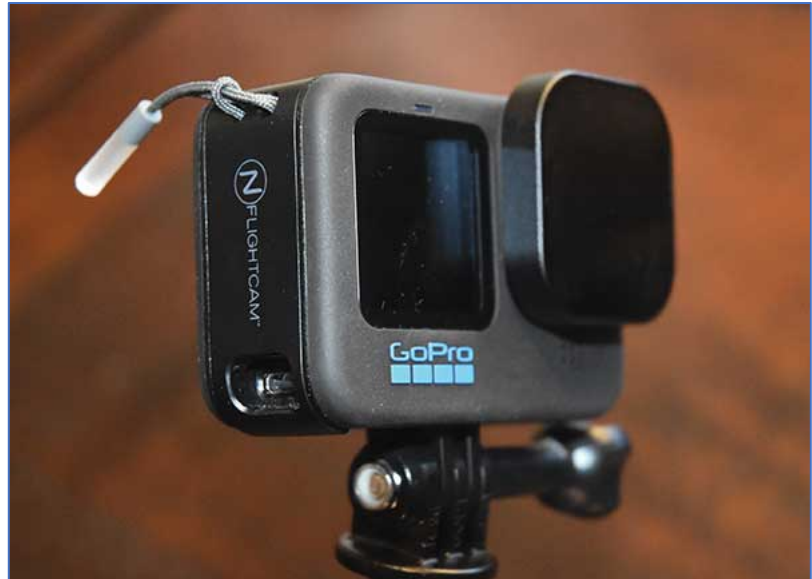
Two clever upgrades on one GoPro 10 camera. First, the rectangular prop filter covers the normal GoPro lens and eliminates from your videos the distracting, swirling prop "scimitar" which is an artifact of the shutter speed and the prop RPM. This is very handy on single-engine aircraft where forward-looking camera shots are always through the prop. On the left side of the camera notice the NFlightCam replacement battery cover. This hatch voids the waterproofing of the GoPro 10, but allows access to the micro-USB port. With access to that port you can power the camera or record intercom audio, depending upon the cables you employ.
