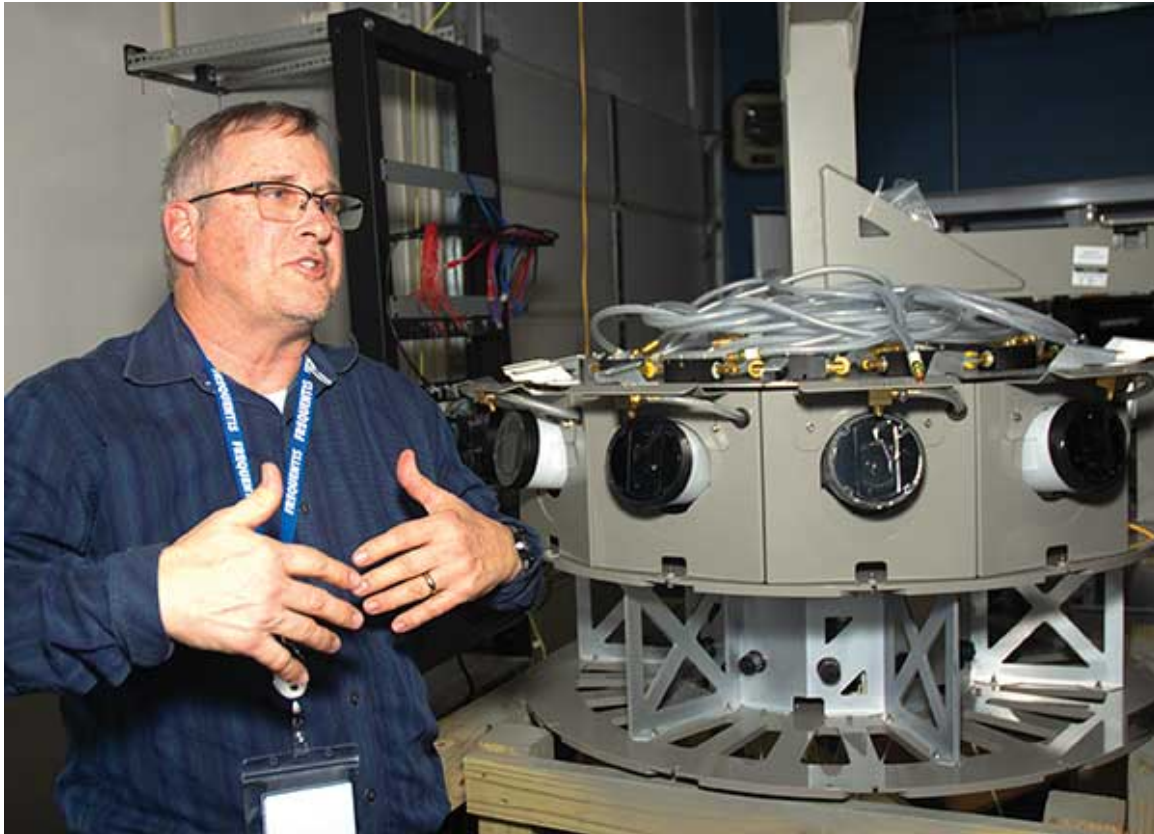
Tim Arnett is the project leader on the remote digital tower technology for Frequentis. On his left is a typical camera installation for an airport, showing the eight primary cameras. The housing has been designed for sixteen cameras, and the additional eight are back-up systems. Each camera comes with a lens cleaning system to keep snow, ice, dust, or pollen from degrading the imagery.
