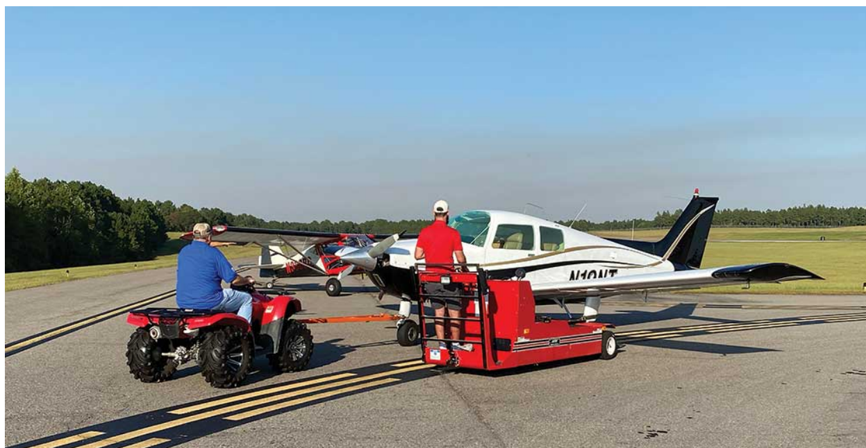
The scene of J.P.'s flat tire. The recovery was a tricky operation because the airport's normal runway-clearing crane was out-of-action for maintenance. Slim Thompson, in the blue shirt, devised a plan where two tugs operated simultaneously. One tug lifted the flat tire off the pavement while the other tug moved the plane. Keeping their positions synchronized during turns was quite a ballet. Notice the author's red Bushcat taildragger on the taxiway, behind the Sundowner.
