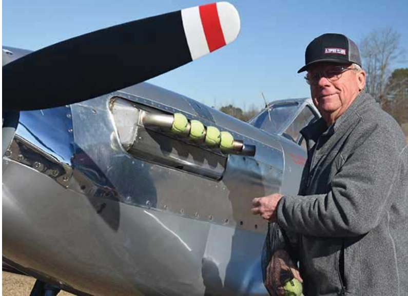
Photo 3: Ben Burril arrived in his miniature P-51, performing a snappy pirouette into parking. He plugs the exhaust pipes with tennis balls to keep FOD out of a very expensive engine.
