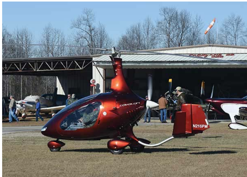
Photo 4: Barry Kropelin brought his Cavalon Autogyro, a gyroplane with side-by-side seating. With a ROTAX engine and available Garmin avionics, this is an exotic but practical flying machine. Photo Credit: Savannah Ritch.
