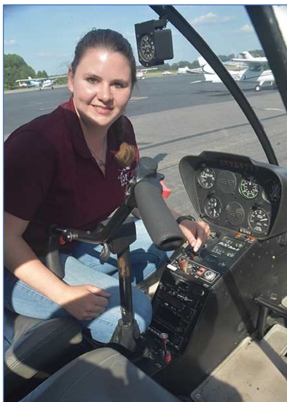
A helicopter cockpit features an alarming amount of glass and a scary lack of instrumentation. A helicopter pilot uses four controls simultaneously to stay in the air: the cyclic down by each pilot's side, the collective, a throttle mounted on the collective, and anti-torque pedals under each foot. Just to make things really special, a helicopter PIC always sits on the right side of the aircraft.
