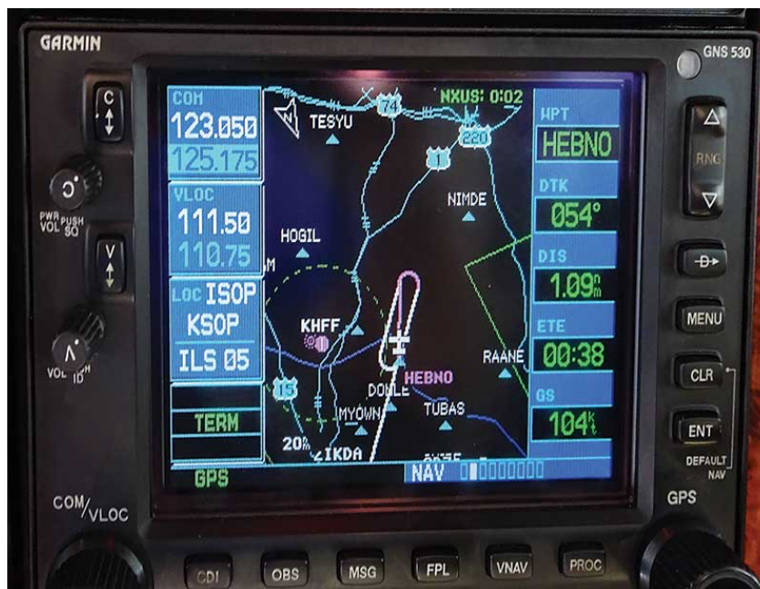
The GFC500 flies marvelously. On a very hot and very bumpy summer afternoon, with density altitude over 2,000 feet, the Garmin comfortably maneuvered old '91N over to the initial approach fix of the ILS-5 at Pinehurst Airport (KSOP). The Garmin 530W shows the plane flew the procedure turn and zipped down the ILS to minimums. (Yes, I switched from GPS navigation to the localizer when the procedure turn was completed.)
