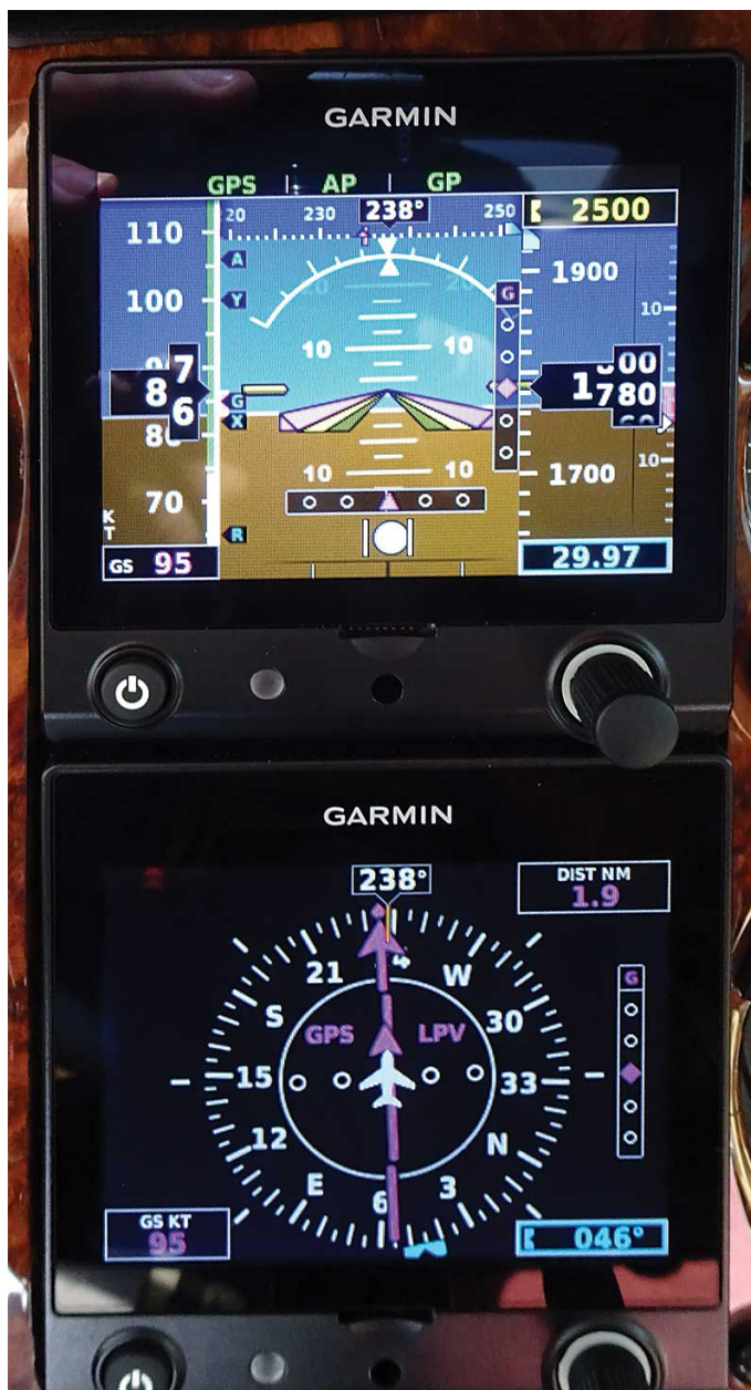
Here’s another instrument approach, displayed on the dual G5s. The plane has just crossed the initial approach fix on the LPV-23 at KSOP and I have activated the APR (approach) mode on the GFC500. The Garmin flight director (top) offered horizontal guidance (the magenta triangle inside the black bar at the bottom of the display) and vertical guidance (the magenta diamond on the black bar on the right side of the display). The lower display presented that same information in a more traditional HSI format. All the captain needs to do is adjust the power, lower the gear and awake up the co-pilot.
