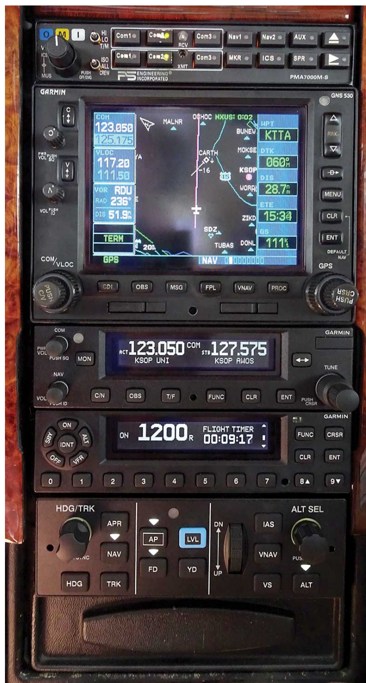
Here's the latest iteration of the avionics stack in Centurion 91N. At the top is a PS Engineering audio panel which has served very capably for nearly two decades. The Garmin 530W is the principal navigator, followed by a new Garmin nav/com radio and the ADSB in-and-out Garmin transponder. The GMC507 control head completes the set. Notice the black plastic spacer at the bottom of the stack — these new systems are far smaller, lighter, cooler and less energy-hungry than the older designs
