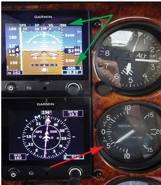
The software elves at Garmin jammed an enormous amount of information into the small G5 digital displays. The top instrument is an integrated flight director while the bottom gauge is a digital HSI. The green arrows highlight my command to the G5 autopilot to descend at 500 fpm. The red arrow shows the old analog gauge agrees with the computer exactly. In all the cross-comparisons I have tested, the digital and analog instruments matched perfectly.
