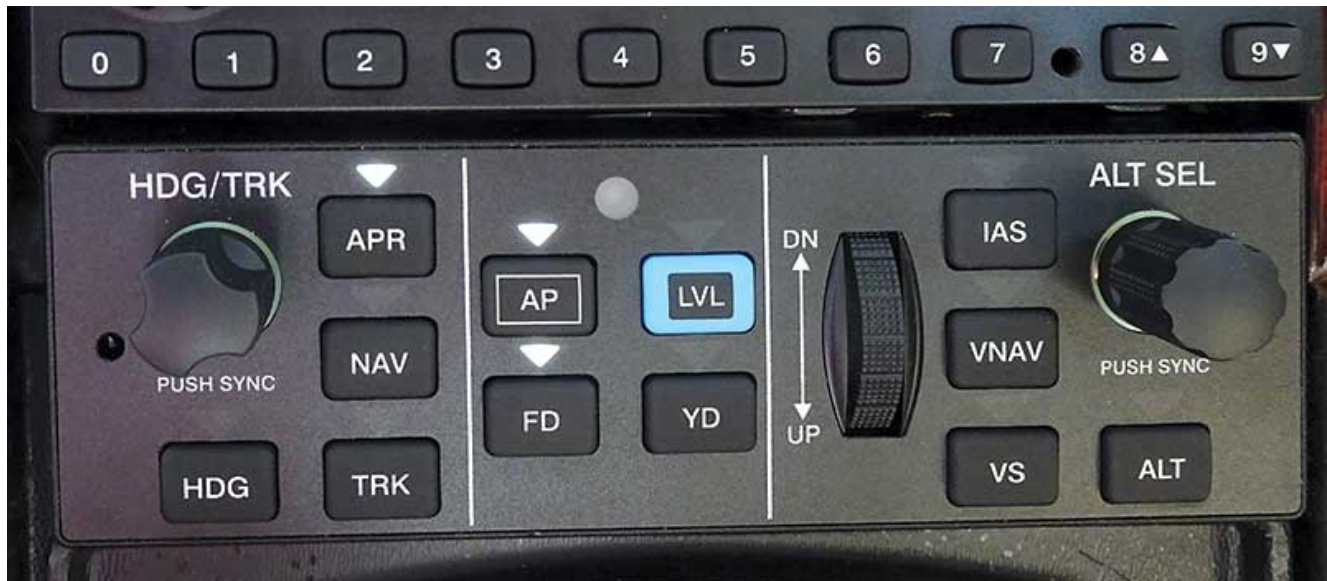
The GFC500 control head is the GMC507. It uses excellent ergonomics to maximize safety and performance. It offers a variety of controls and options including "Approach Mode" which can automatically intercept a localizer and a glide slope and fly right to minimums.
