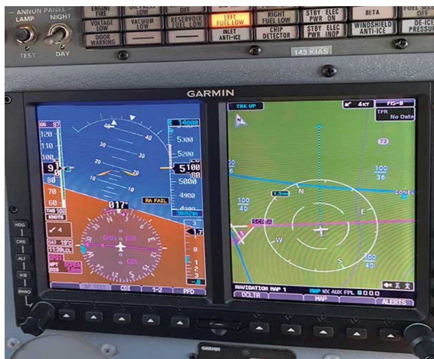
The Caravan is perfectly equipped for skydiving. The left display shows Ribbeck is at 5,100 feet and 91 knots, in a gentle left-hand turn to track towards the drop zone. He's climbing at 3,000 fpm. The right display shows the magenta track towards the drop zone, which is located on the eastern edge of the runways at Chester Airport (white triangle, left). Ribbeck minimizes wasted time or fuel by arriving exactly at 14,000 feet at the drop zone. Notice the “low fuel” alarm.
