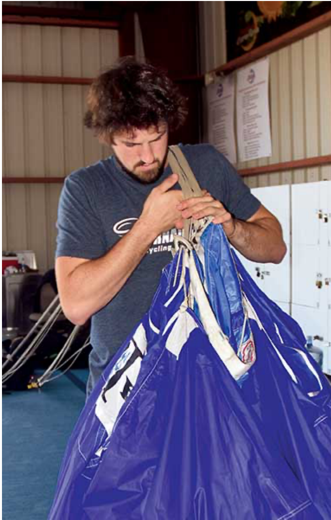
Eli Hyatt has been a professional rigger for six months. Here he's smoothing the rigging lines that connect to the cells of the parachute. He then folds and smooths each cell by wrapping them around his torso.
