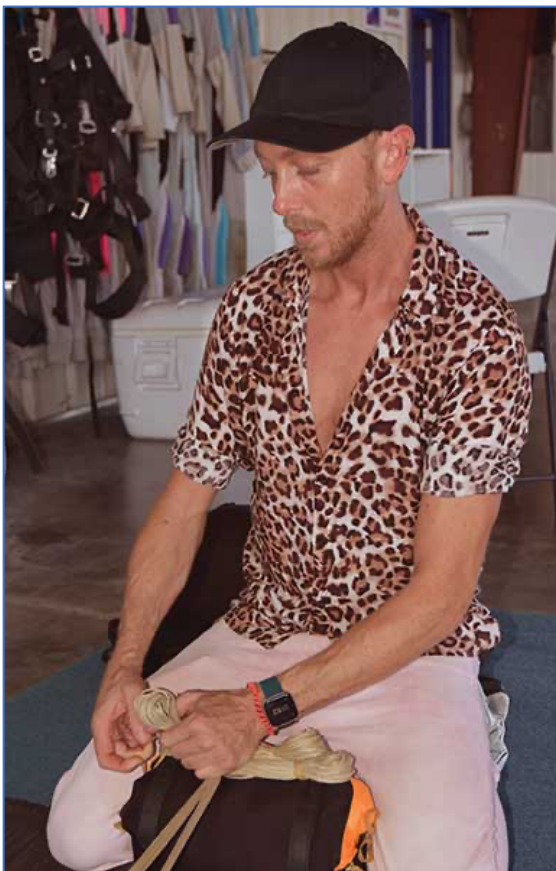
Jake Herring uses fat rubber bands to hold the lines in the proper position before stuffing everything into the parachute case. Herring has been packing chutes for more than two decades and spoke knowledgeably about different techniques, canopies and procedures. His professionalism and confidence was reassuring.
