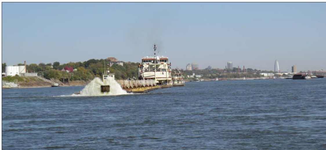
Seven dredges moved nine million cubic yards of material at 70 different locations along 300 miles of river channel in the US Army Corps of Engineers' St. Louis District in 2022. A normal average is three to four million cubic yards with just two dredges working. Photo courtesy of USACE, photo by Janet Meredith.
