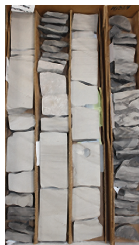
Vogelsang 1 core showing interbedded sandstones and shales, passing upwards to laminated sandstones (part of a delta front succession)
