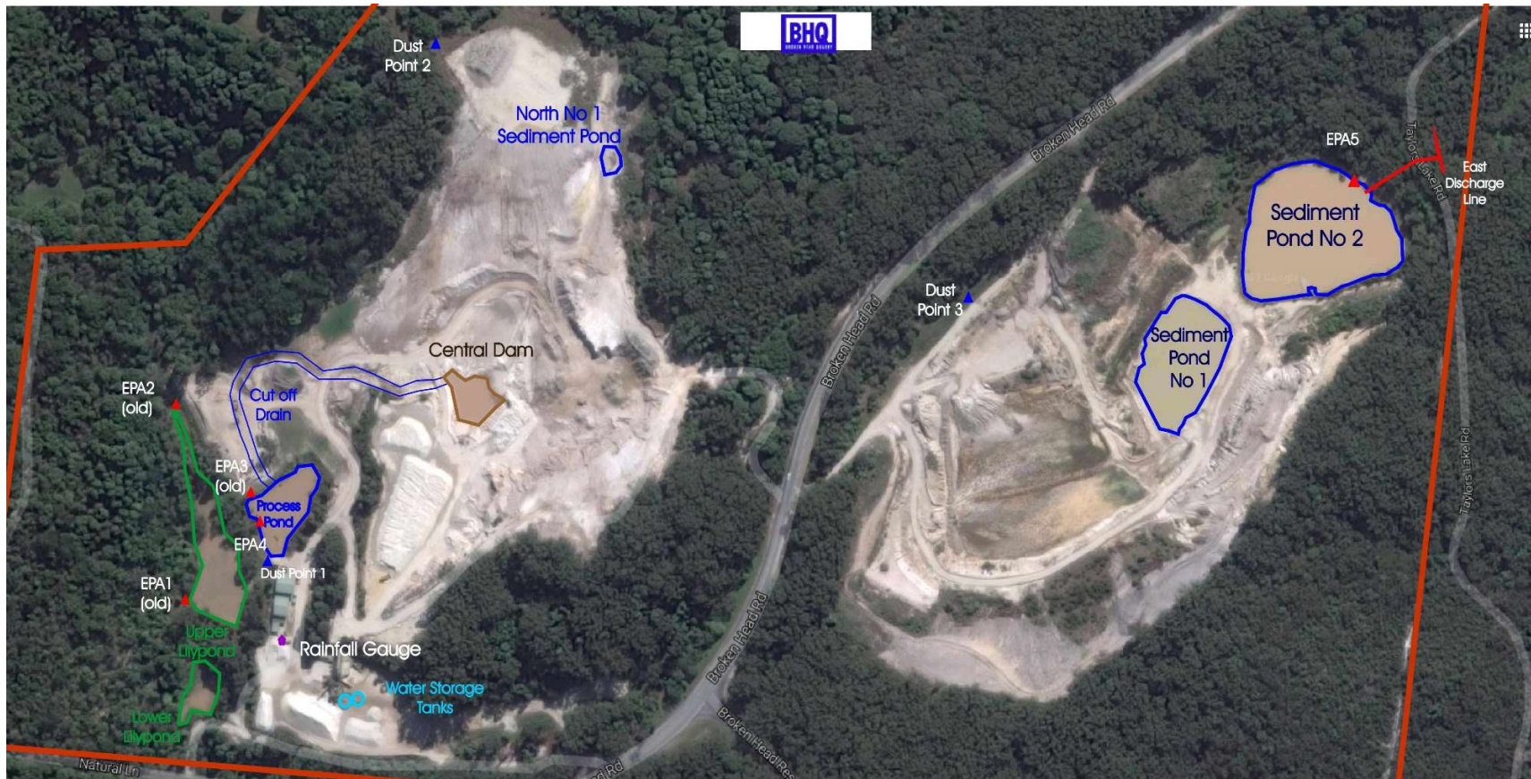
Figure 1 – Plan of major features of Broken Head Quarry
