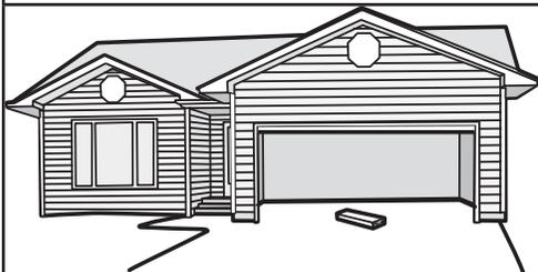
Press the remote control push button to close the door. The door MUST reverse when it makes contact with the board.
