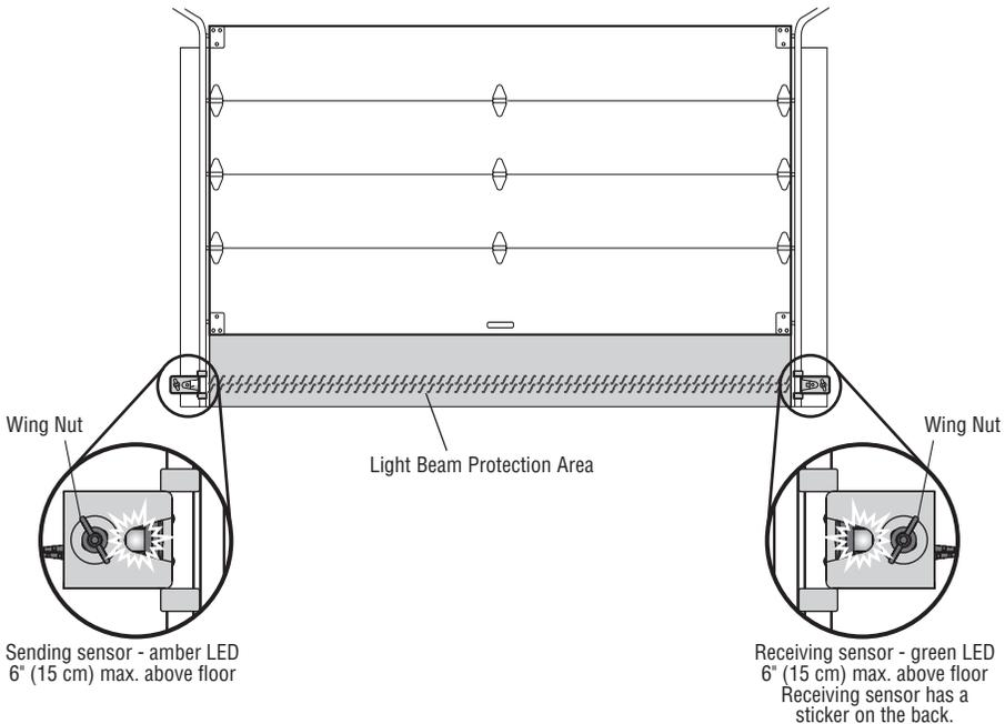
**If either of the sensor LEDs are off, there is no power to the sensor:**
