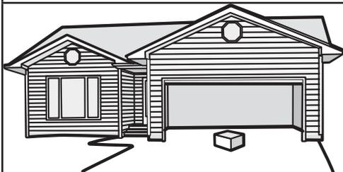
Press the remote control push button to close the door. The door will not move more than an inch (2.5 cm).
