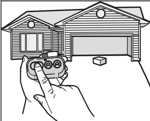
The garage door opener will not close from a remote control if the LED in either safety reversing sensor is flashing (alerting you to the fact that the sensor is misaligned or obstructed).
