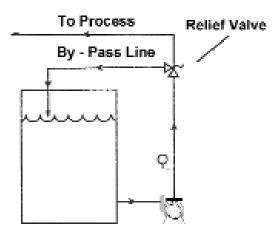
Figure 2: By-pass Configuration
