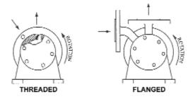
Figure 1: Direction and Port Location
