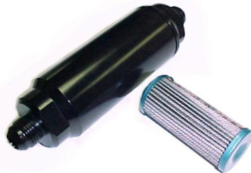
Filter installs directly in the oil line before an external differential or transmission cooling pump. It's 240 micron stainless element suits all oil types, weights and viscosities. Housing- anodized 6061 aluminum 1.75" x 6.25", Element- 304 stainless mesh 1.125" x 2.75" (240 micron) rating, stainless steel support spring (150 psi rated), Viton o-ring seals on end cap, -8AN or -6AN male fluid connections
