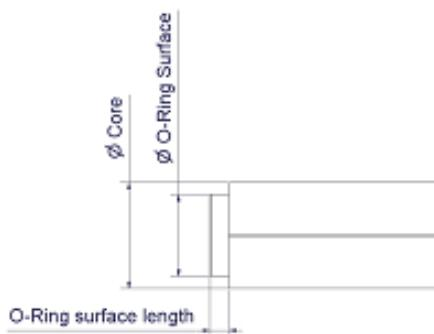
The intercooler core is available in two diameters ø39,5 and ø45.
