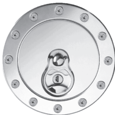
Aero 500 Cap cap: 4.0" cap material: 6063 Aluminum flange material: 6082T6 flange bolt circle: 4.75" PCD fixing holes: 12 x 5mm mounting: flush flange (direct) or for (remote) mounting use funnel/neck 3.5" hose versions: locking or non-locking
