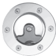
Aero 200 Cap cap: 1.75" cap material: 6063 Aluminum flange material: 6082T6 flange bolt circle: 2.5" PCD fixing holes: 6 x 4mm mounting: flush flange (direct) hose flange 2.0"(remote mount) versions: non-locking only
