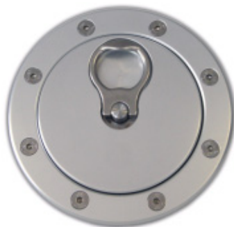
Aero 600 Cap cap: 3.5" cap material: 6063 Aluminum flange material: 6082T6 flange bolt circle: 4.25" PCD fixing holes: 8 x 5mm mounting: flush flange (direct) or for (remote) mounting use funnel/neck 2.0" hose versions: locking or non-locking
