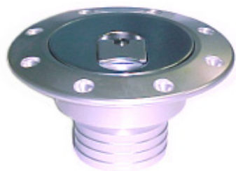
Aero 400 Cap cap: 3.0" mounting: (remote) mounting use funnel/neck 2" hose to tank. versions: locking or non-locking
