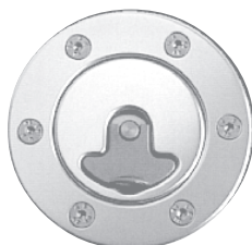
Aero 300 Cap cap: 2.25" cap material: 6063 Aluminum flange material: 6082T6 flange bolt circle: 3.0" PCD fixing holes: 6 x 5mm mounting: flush flange (direct) or step flange 2.25"/2.0"(remote) versions: locking or non-locking
