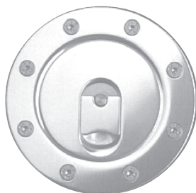
Aero 400 Cap cap: 3.0" cap material: 6063 Aluminum flange material: 6082T6 flange bolt circle: 4.0" PCD fixing holes: 8 x 5mm mounting: flush flange (direct) or for (remote) mounting use funnel/neck 2" or 2.25" hose versions: locking or non-locking
