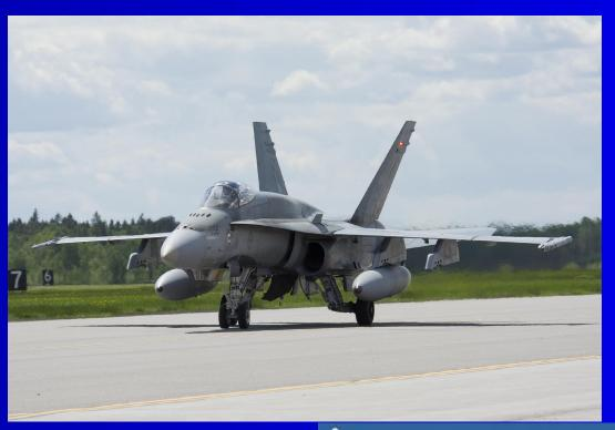
Skinny wings provide lift at high speeds with less drag. However, they are more prone to stall.
